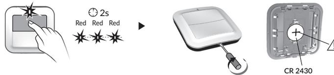
The red LED flashes each time you press = Battery fault
