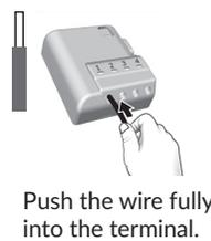
Push the wire fully into the terminal.
