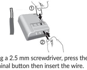
Using a 2.5 mm screwdriver, press the terminal button then insert the wire.
